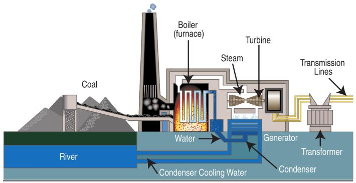
Note: Diagram of essential components of a coal fired power plant
